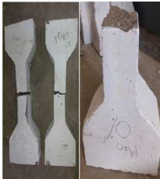
Fig 5.1 Failed specimen and fractured surface
